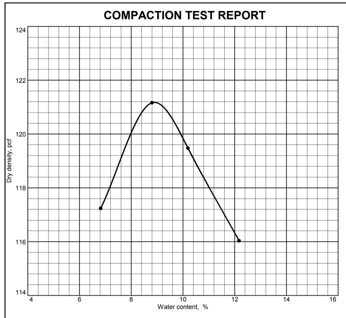
Test specification: ASTM D 1557-12 Method A Modified
