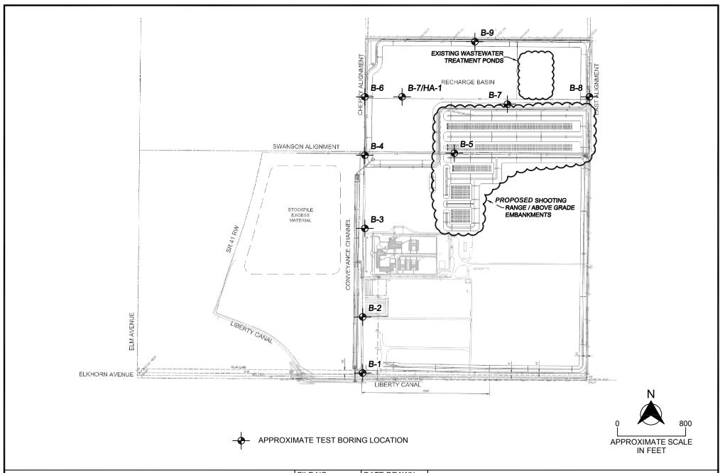
TEST BORING LOCATION MAP ELKHORN RECHARGE PROJECT NORTHEAST OF INTERSECTION OF ELKHORN AVENUE AND HIGHWAY 41 FRESNO COUNTY, CALIFORNIA
