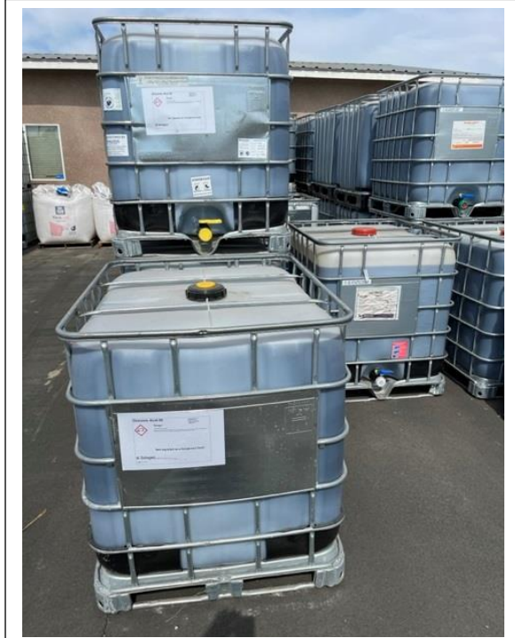
Outdoor storage of finished materials in 275-gallon totes with DOT label.
