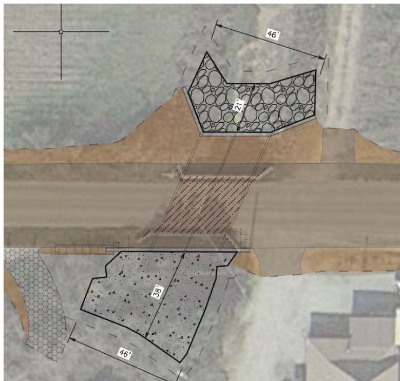
Figure 3 Rock Slope Protection and Concrete Channel Lining
