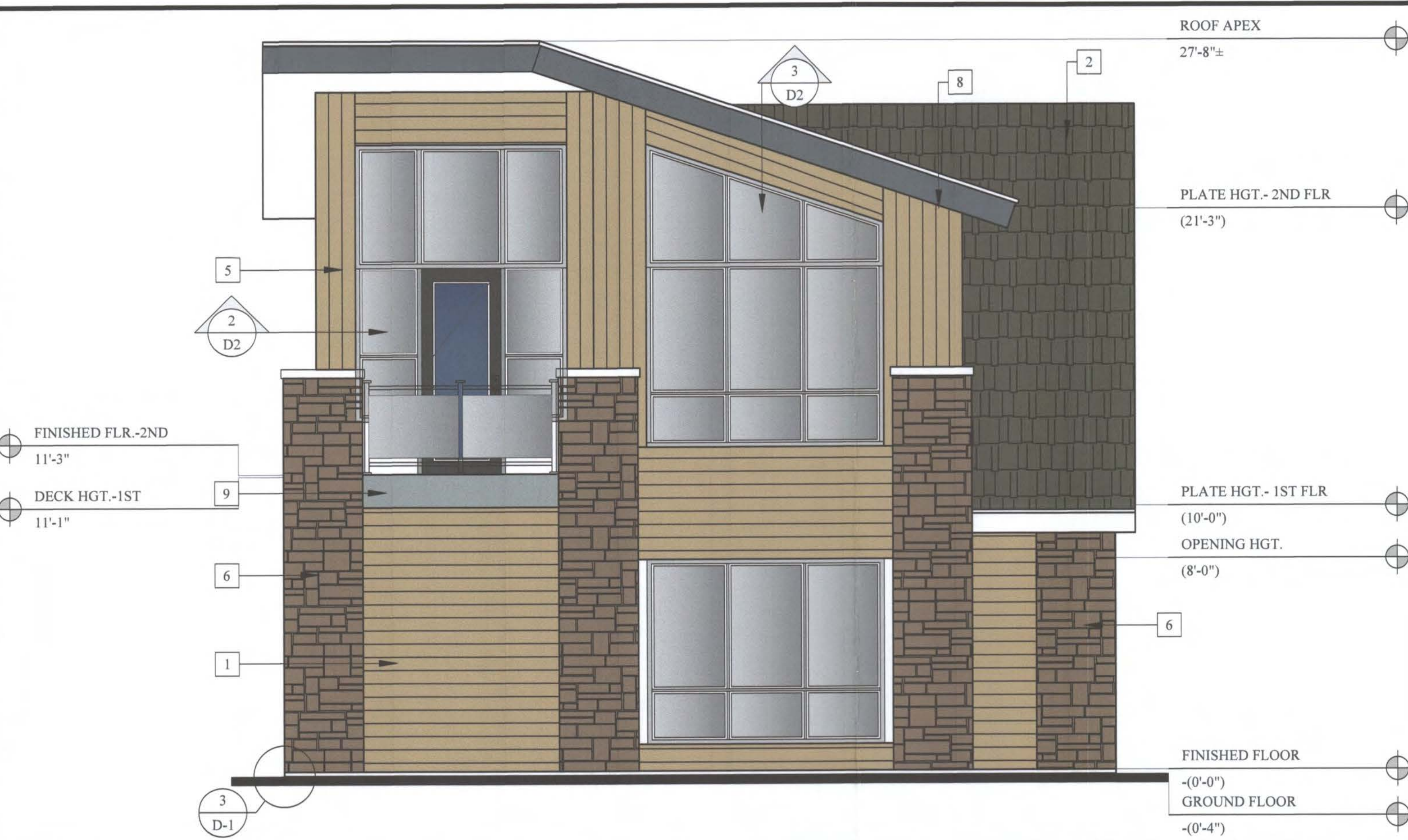
FRONT ELEVATION - NORTH SCALE - 1/4" = 1'-0"
